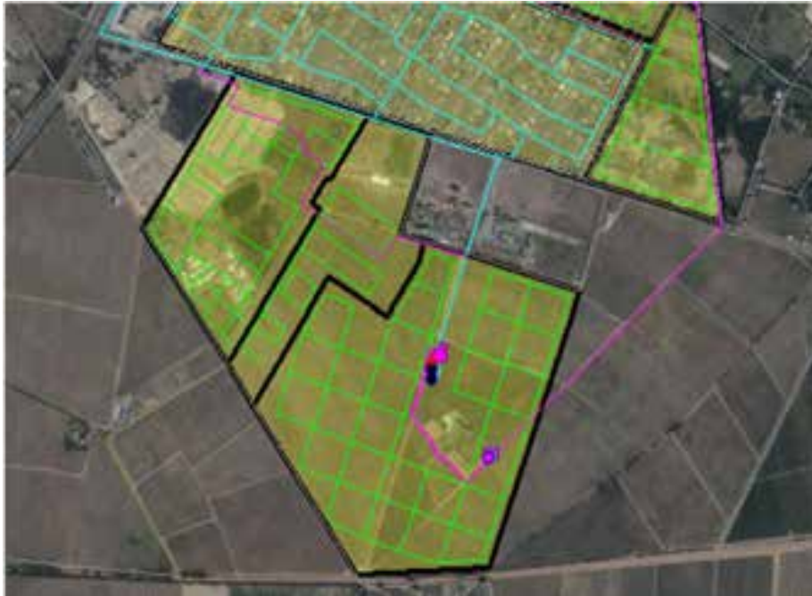
Figure 4: Jamestown - Master Plan Water Distribution System
