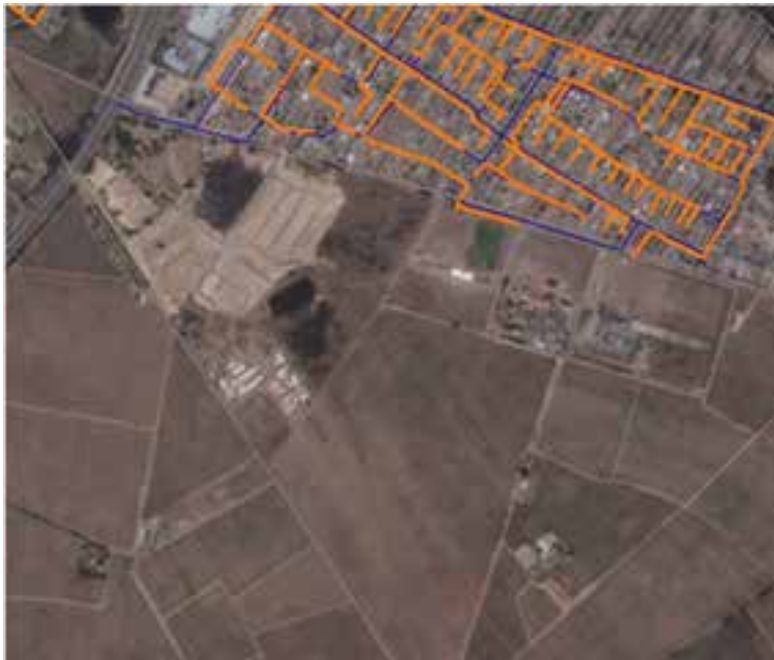
Figure 5: Jamestown - Detail Master Plan Water Distribution System
